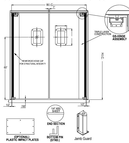
Doors are constructed of a 1/2" thick polyethylene H.D.P.E. sheet. Standard features are:
